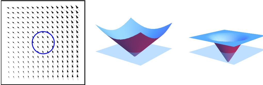
Figure 2–14: Level set modification for a flow crossing boundaries. The left figure shows the case of a circle transported in a vector field that enters and exits the domain. The middle figure shows the level set function we would usually use, and the right figure shows a modified level set function that is constant around the boundary, allowing it to be evaluated outside the domain through trivial extrapolation.
